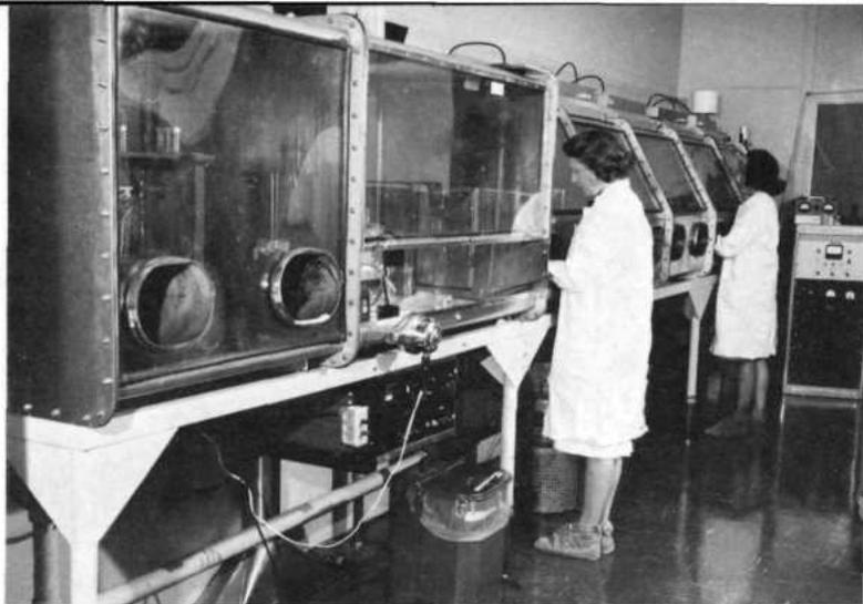
*A glove-box train used in preparing metallographic specimens containing plutonium. An analytical balance for weighing specimens is visible in the glove box at the left. Specimens are brought into the train through the open front hood (second enclosure from the left), and a variety of operations (cutting, filing, grinding, polishing) are performed in the boxes at the right.*
